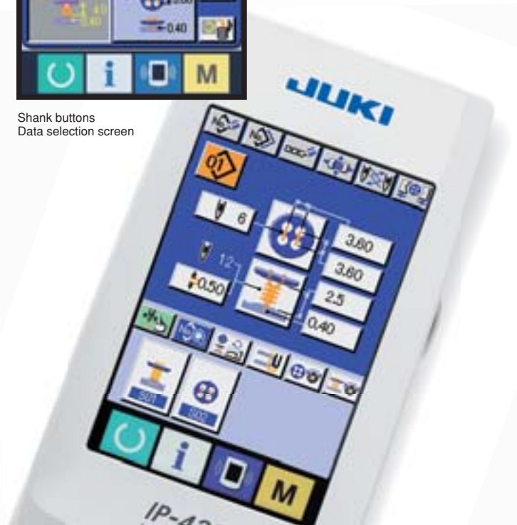
Setting of longitudinal and lateral adjustments of button chuck.
